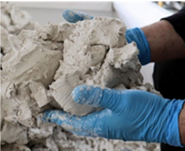
(174) Fanghi di natura marmorea (Fonte: A Novel Approach for the Reuse ofWaste from the Ex- tractive and Processing Industry of Natural Stone Binders: Development of Stone Composites - pp. 6)
