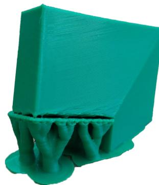
Fig. 4.3 – Example of PLA external supports created by the 3D-printing machine.
