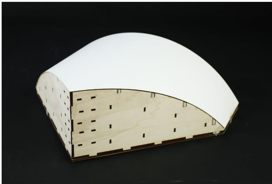
*Fig. 4.12 – Final plywood prototype, assembly process of the centering system. Single web.*
