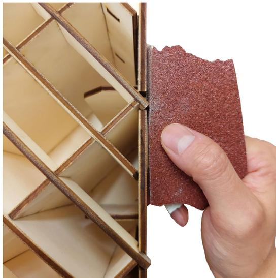
*Fig. 4.10 – Final plywood prototype, manually sanding the ends of small arches.*
