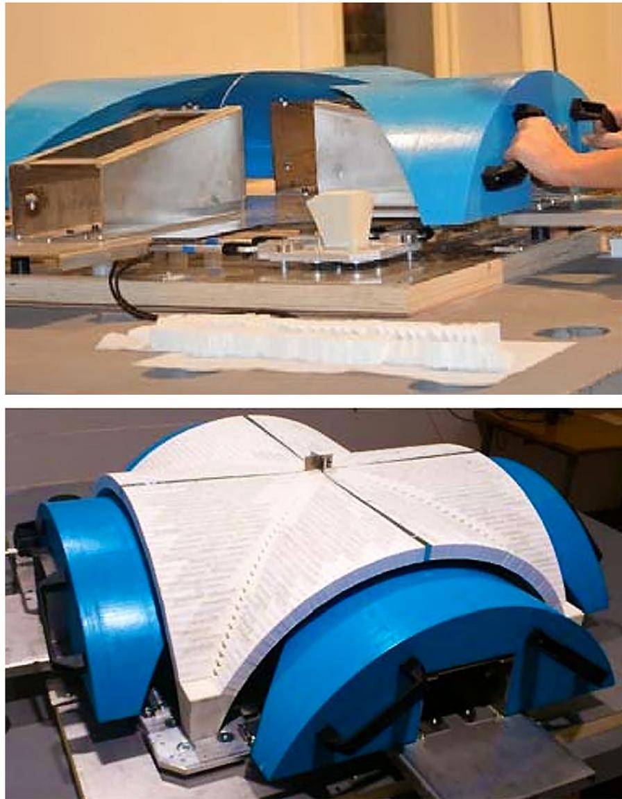
Fig. 1.3 - Testing setup for small-scale cross-vault, focus on the centering system (From: Rossi 2015 [4]).
