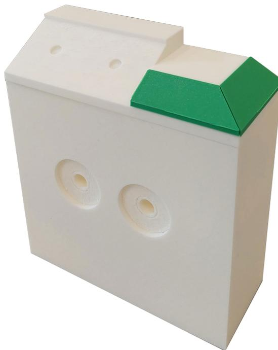
*Fig. 4.4 – 3D-printed prototypes of the cross-vault abutments. The green parts represents the plates described in Figure 3.11; although they will be printed using the same material as the vault blocks, they were printed at this stage to test the functionality of the interlocks with the underlying part.*
