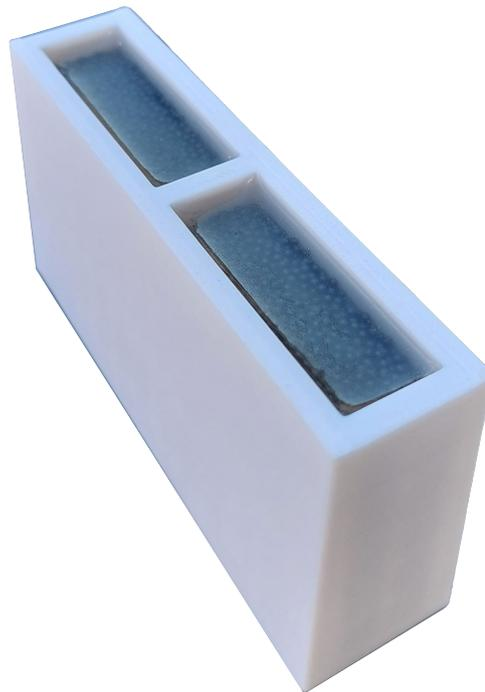
Fig. 4.2 – Head arches blocks: 3D-printed via FDM and filled with led pellets and epoxy resin.
