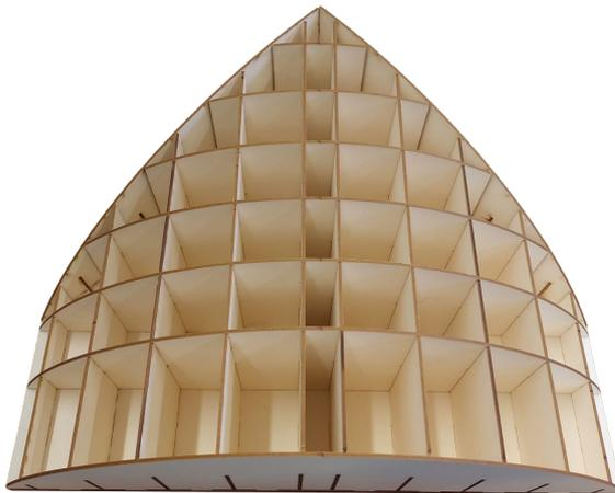
Fig. 4.5 – First prototype in carton bois, assembly test. From the top: diagonals; longitudinal diaphragms; transverse diaphragms; first arched diaphragm.
