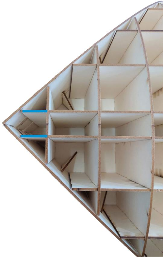
*Fig. 4.6 - First prototype in carton bois, main issues. Instability of the apex, lack of support in relation to the diagonal diaphragms.*
