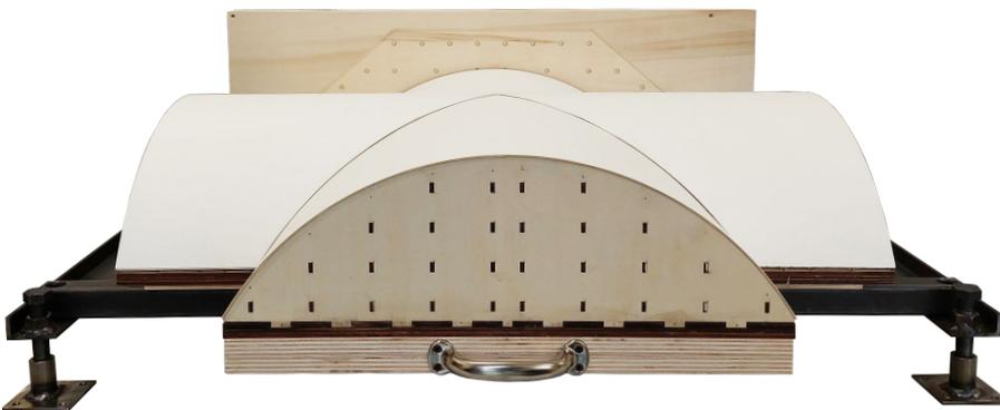
*Fig. 5.2 - Prototyped components of the testing setup system. From the top: the steel frame system for moving the plywood centering, assembled components of the testing setup, lateral view and frontal view.*
