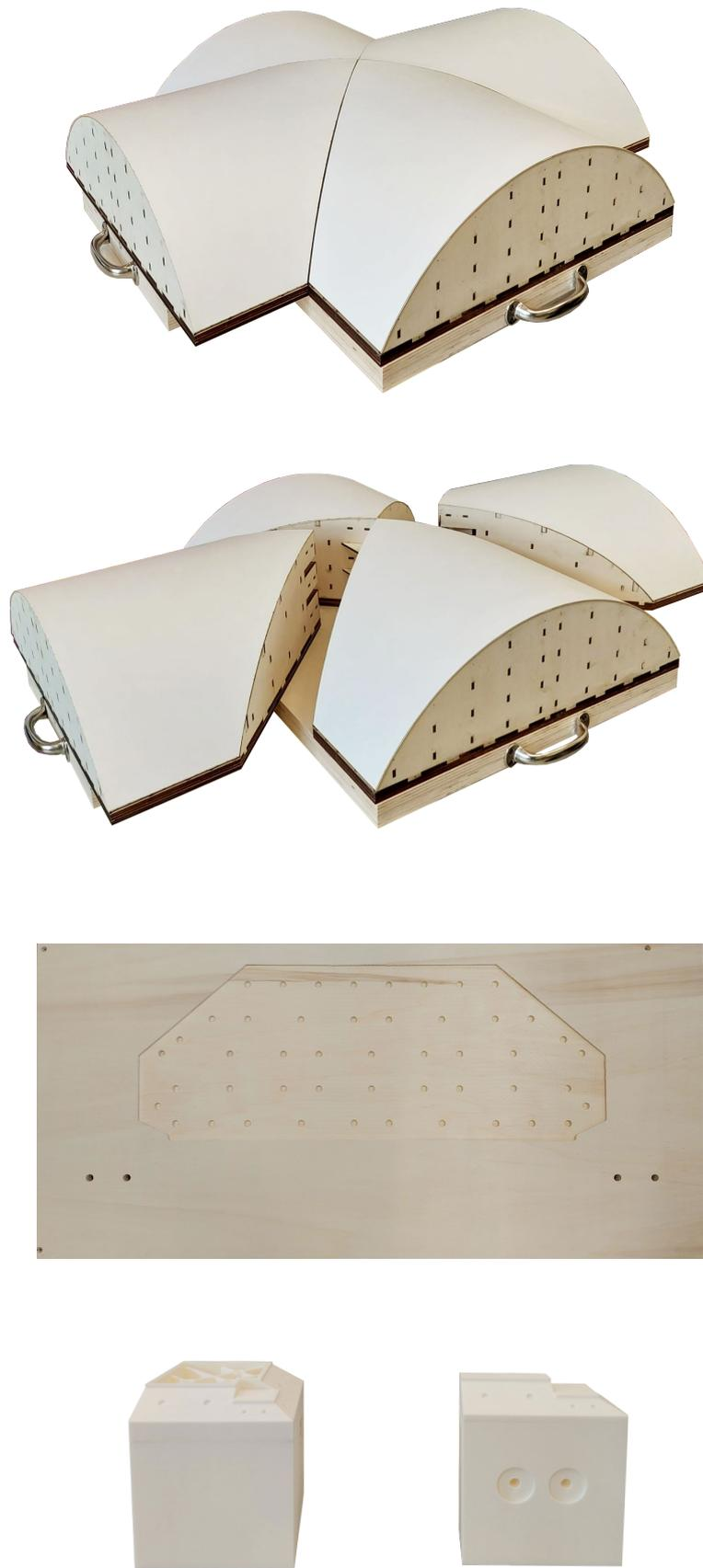
*Fig. 5.2 - Prototyped components of the testing setup system. From the top: plywood centering system, plywood back wall (932 x 450 x 18 mm) realized with a CNC milling machine, vault's 3D-printed abutments.*
