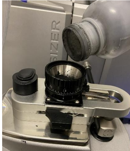
Image 124 Introducing biochar powder particles into the conical steel cell for granulometry analysis
