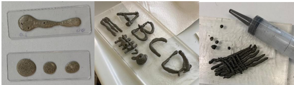
Image 23 Syringe test physical behavior results showing the evolution and variation of the mortars workability by creating different mis design formulations. Source: (Author)
