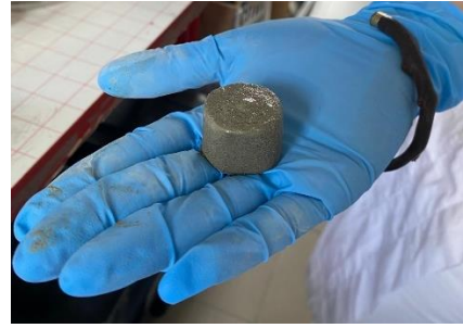
Image19 Mortar paste after undergoing the syringe test without success as it lacked workability. Source: (Author)
