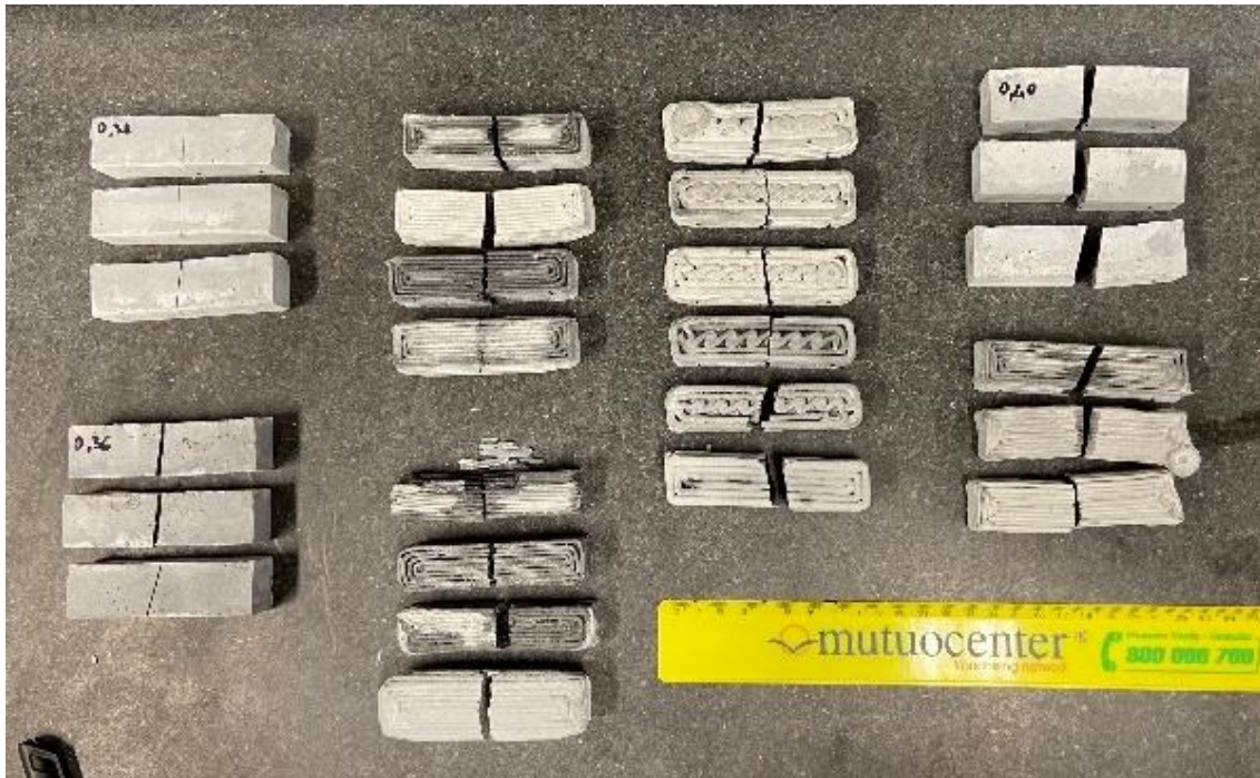
Image 48 Arrangement of the fractured halves of the mortar prisms from the flexural tests, prepared to begin the compression test. Source: (Author).
