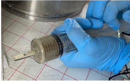
Image18 Simulation of the 3D printer extrusion with a 5mm syringe. Source: (Author)
