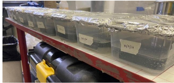
Image 39 28-day mortar sample hydration. Source: (Author)
