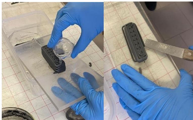
Image 38 Unmolding process of 3D printed samples.
