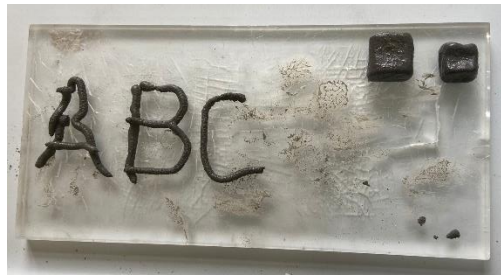
Image 22 Syringe and moldability - physical behavior mortar mixture design test results. Source: (Author)
