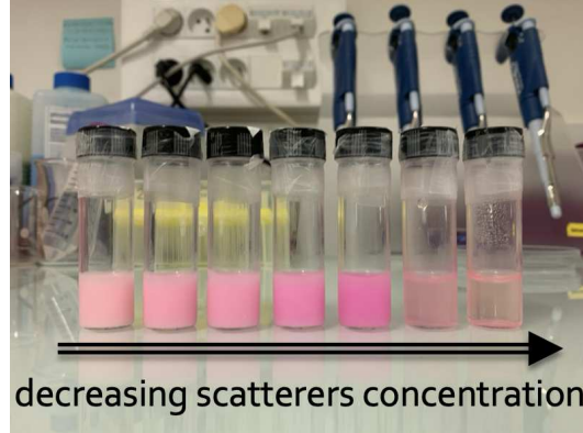
Figure 3.4: Samples from P300R20 to P1R20 , where the concentration of rhodamine is fixed at \rho = 5.36 \cdot 10^{21} molecules/m 3 and one of beads varies from a maximal one of \rho_s = 9.69 \cdot 10^{17} beads/m 3 (left-most) to a minimal one of \rho_s = 3.23 \cdot 10^{15} beads/m 3 .
