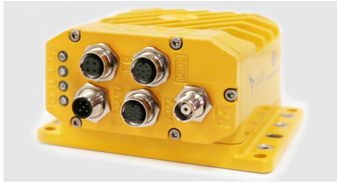
Figure 5.2: Swift Duro GNSS receiver by Carnegie Robotics [10]
