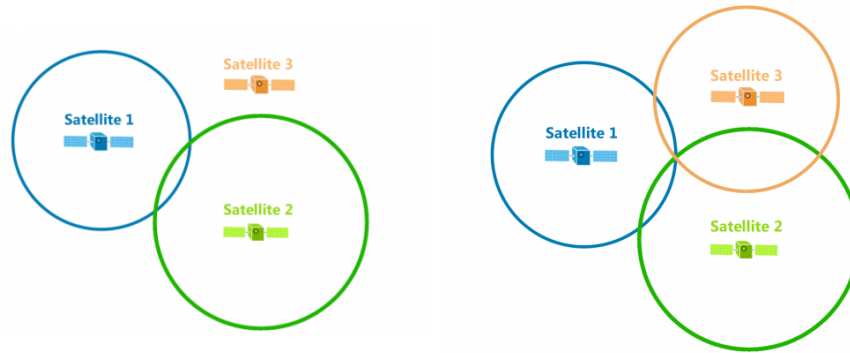
Figure 2.4: Satellite trilateration in 2D. The intersection of two satellite measurements (left) and the intersection of three satellite measurements (right). [3]
