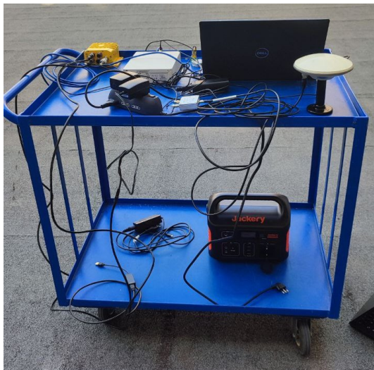
(a) Experimental setup front view with power supply, antenna, RTK device, GNSS receiver
