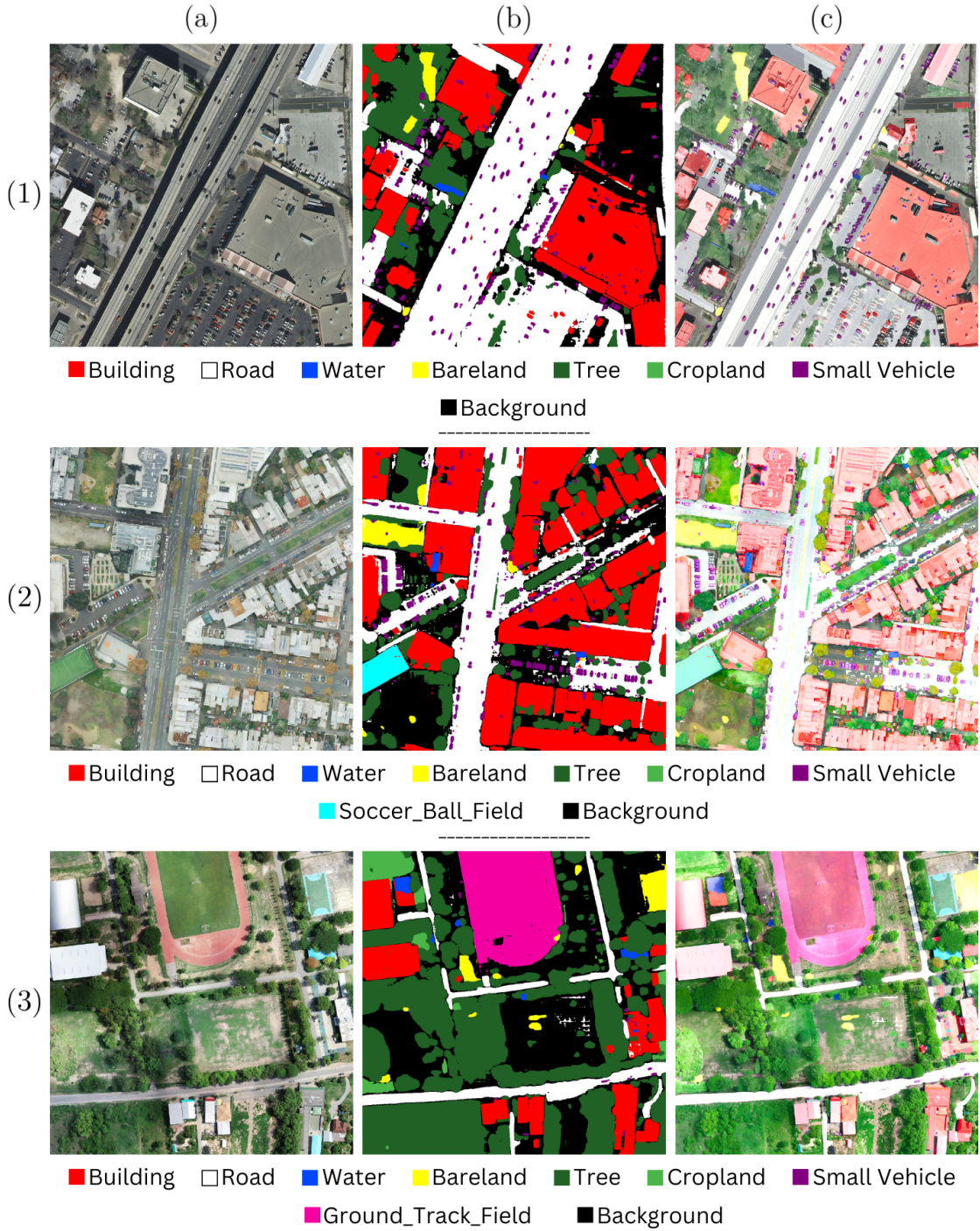
Figure 4.8: Qualitative results of SAM-FC-CLIP along with the text queries and the color used in the visualization. Notable delineated classes are the small cars in purple and some rare categories like the soccer ball field and the ground track field.
