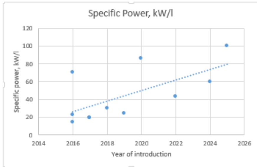
Figure 2: Specific power trend of inverters
