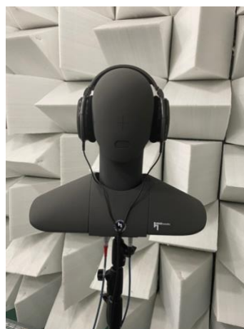
Fig. 31 playback volume adjustment in anechoic chamber
