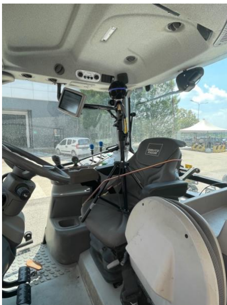
Fig.15 Zylia ZM-1 microphone In the tractor during measurements
