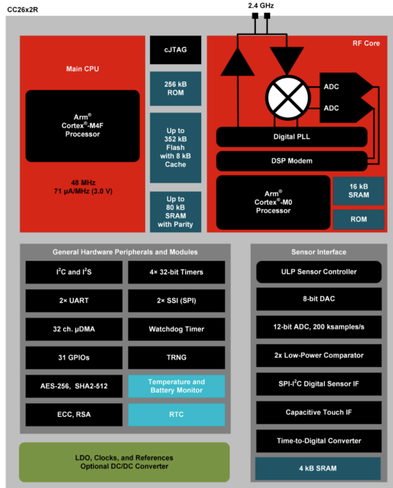
Figure 4.4: CC2652 block diagram
