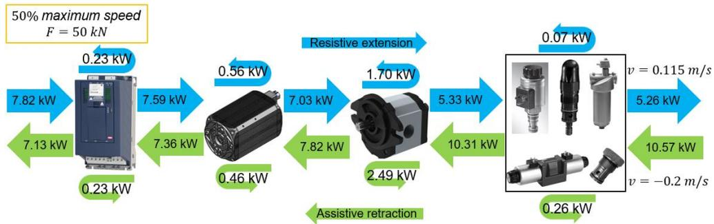
**Figure 6.4: Power flow of open-circuit EHA: 50% actuation velocity command, 50 kN load force**
