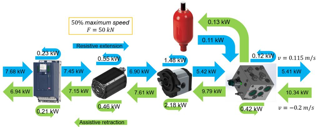
**Figure 6.15: Power flow of closed-circuit EHA: 50% actuation velocity command, 50 kN load force**
