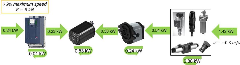
Figure 6.8: Power flow of open-circuit EHA: 75% actuation velocity command, 5 kN load force
