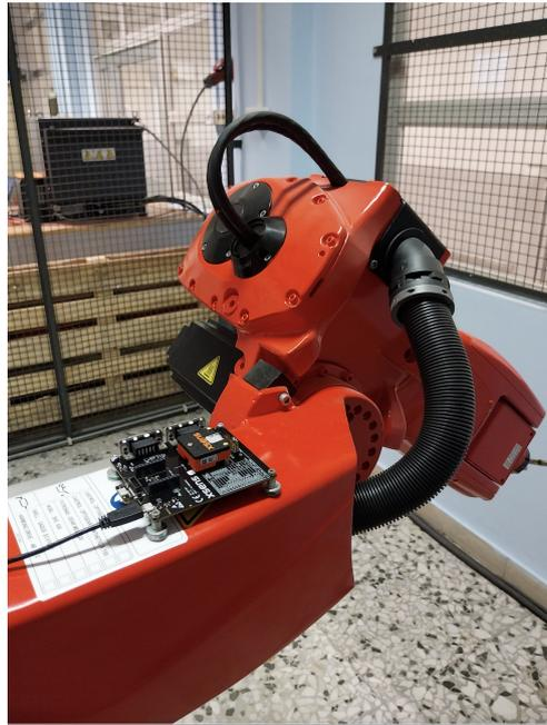
Figure 5.10. Xsens gyroscope above axis 2 of the manipulator
