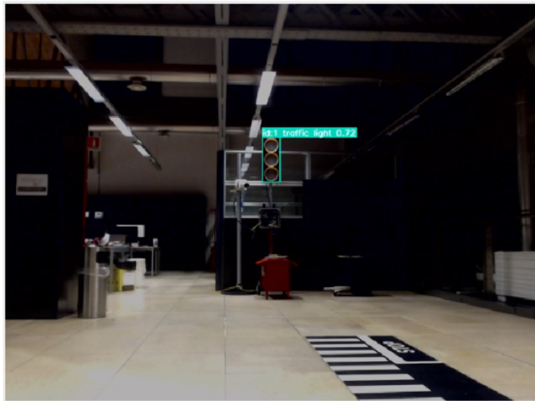
(b) Camera view with YOLO's labeling and bounding box.
