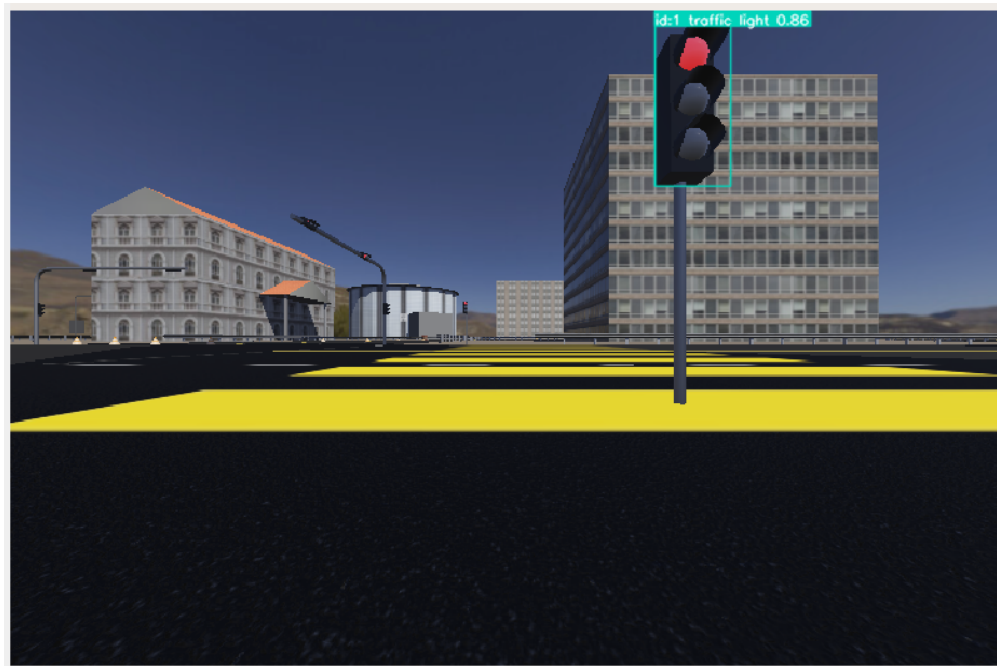
Figure 6.8: RViz2 visualization of the yolo_image topic, with the bounding box and label of the traffic light.
