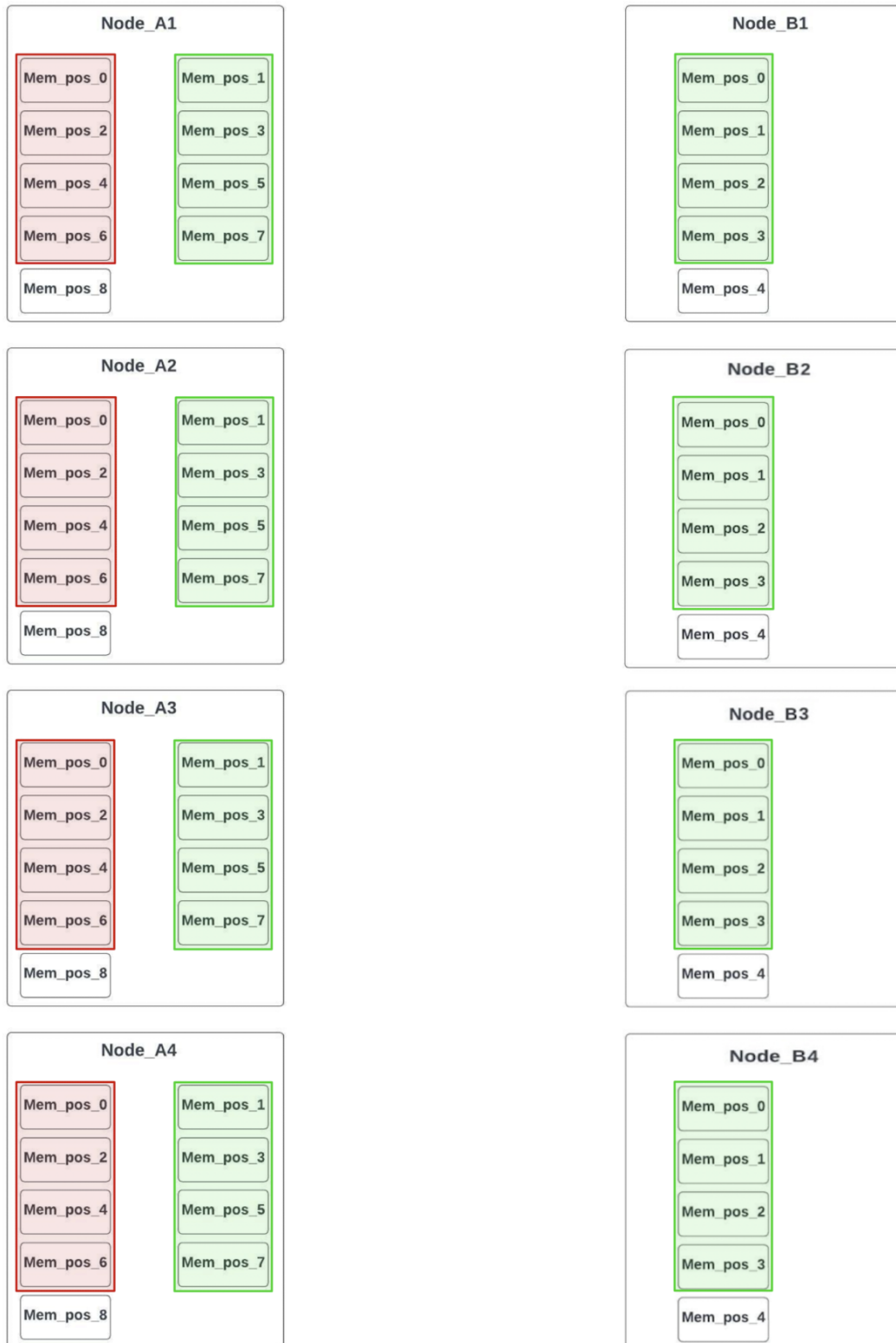
Figure 3.5: Network scheme to show the final memory state after entanglement distribution.
