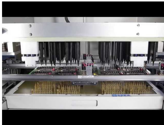
Figure 2.5. Bed of Nails Test Machine 3030
