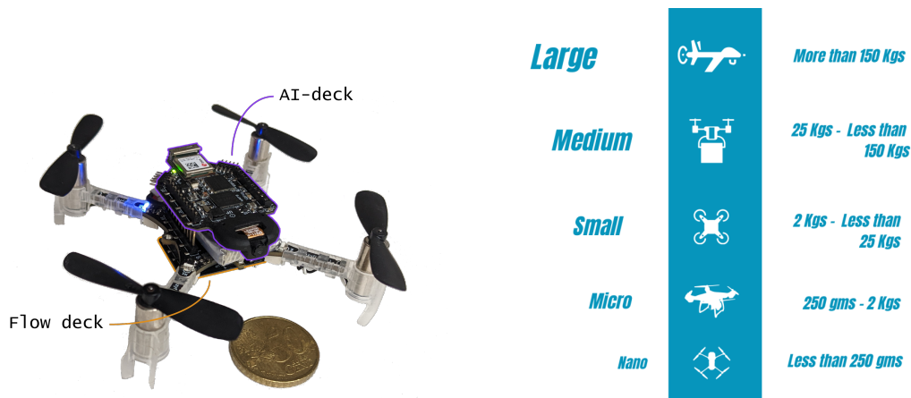
Figure 2.2: Crazyflie 2.1 along with a categorization of UAVs by weight.
