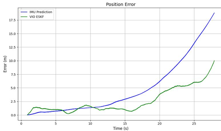
Figure 9.44: Position error comparison between IMU integration and VIO ESKF over time.
