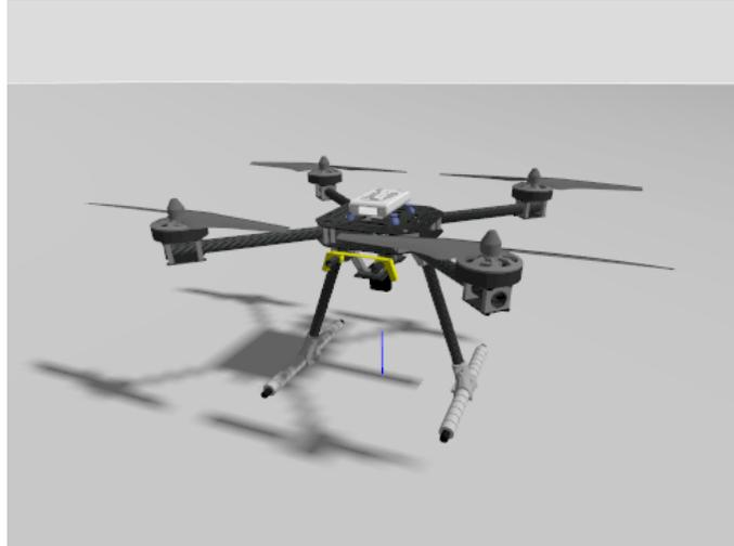
Figure 6.1: X 500 mono cam drone model
