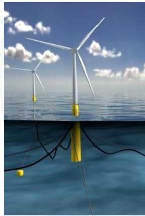
Figure 23: Spar buoy foundation [41].
