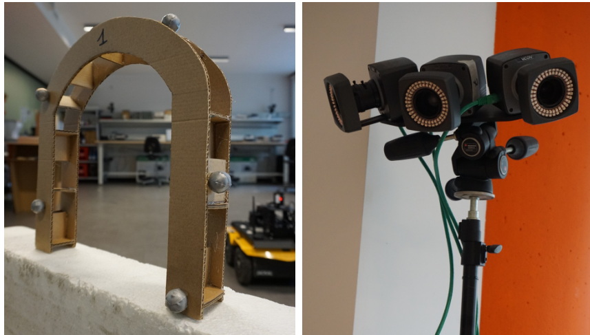
Figure 5.10: One of the U-shaped cardboard frames on the left; three of the ten high-speed infrared cameras of the Vicon® system on the right.
