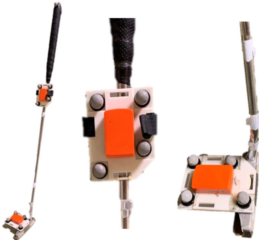
Figure 4.2: Putter equipped with SP markers and IMUs attached to plates.
