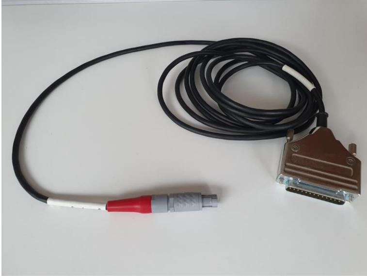
*Figure 24: The g.tec parallel port used to connect the g.Hiamp amplifier to the stimulus computer.*
