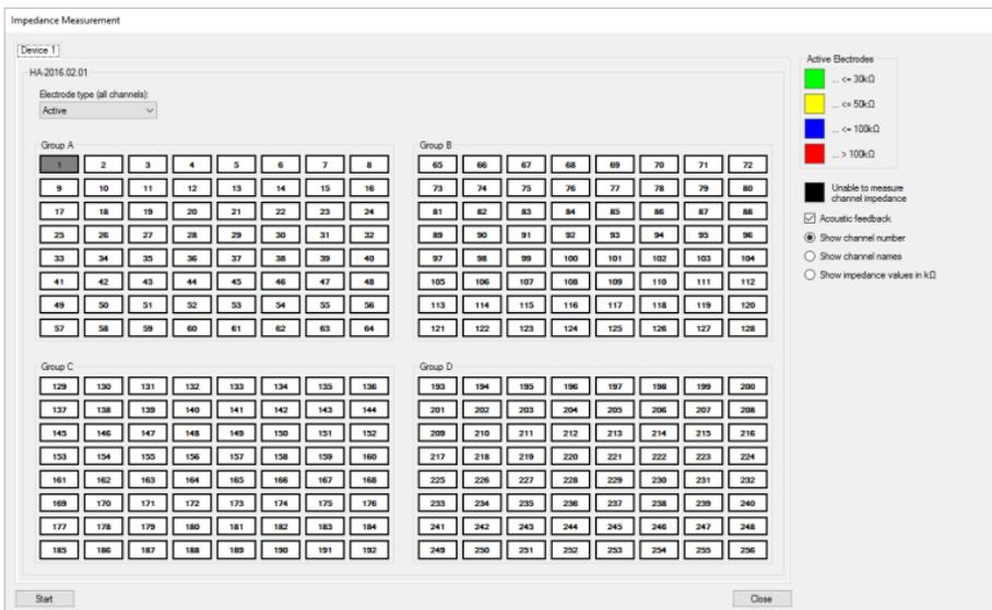
Figure 71: Impedance measurement window on the gRecorder software.
