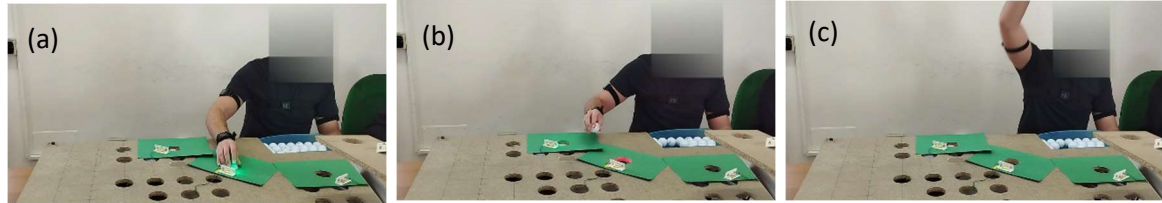
Figure 2.5. (a) Green LED activation: the participant picks up the ball and places it in the designated hole. (b) Red LED activation: the participant moves the ball quickly in a different direction to the hole indicated by the red LED. (c) Buzzer activation: the participant raises their arm vertically as quickly as possible.
