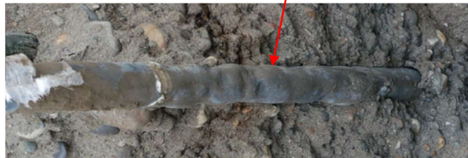
Figure 3.14 –(a) Timpa delle Vigne tunnel face improved by soil nailing;(b) Soil nail bar removed after injection.
