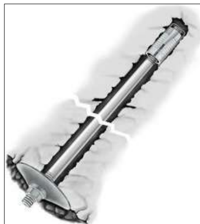
b) Bolts anchored with an expansion sleeve anchor (Reference: Norwegian Rock Bolting (Publication n.21))
