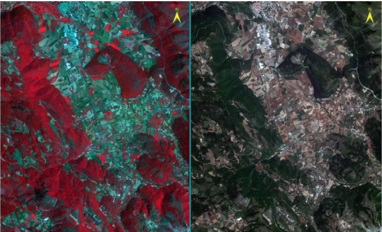
Fig.88 Comparison between False color image (NIR, Red, Green) and acquisition in the visible band (Red, Green, Blue) for the month of July
