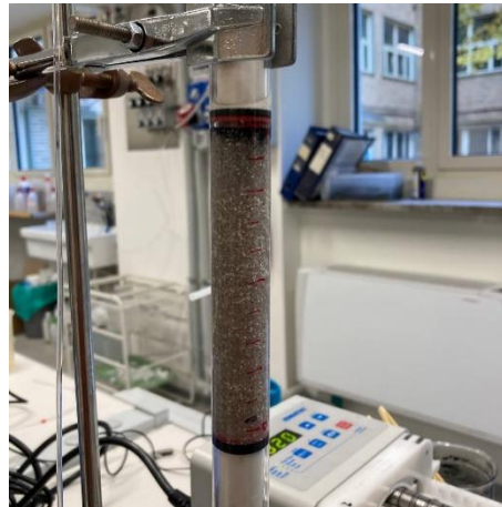
figure 4.28. Final result of column test
