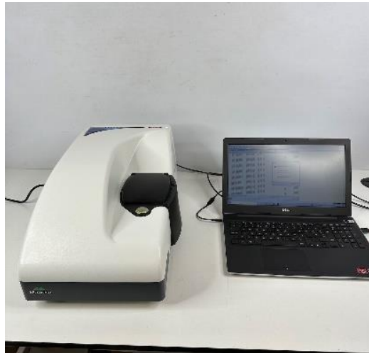
figure 4.3. Zetasizer nano, Malvern Panalytical, Malvern UK (“Malvern Zetasizer Nano ZS ZEN3600 Size and Zeta Potential Particle Size +PC, S/W - SOLD,” n.d.)
