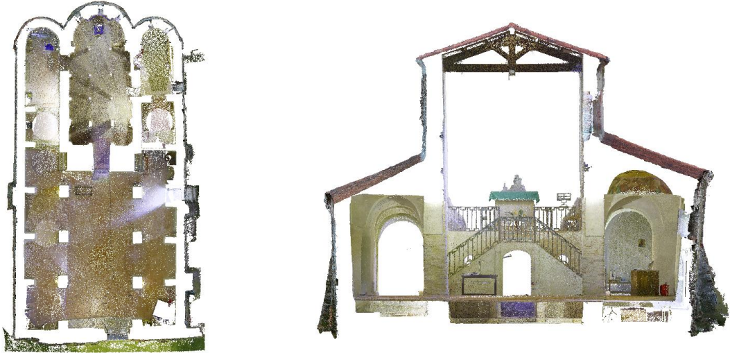
Image 44 - Plan View (left) and Section (right) of the point clouds.
