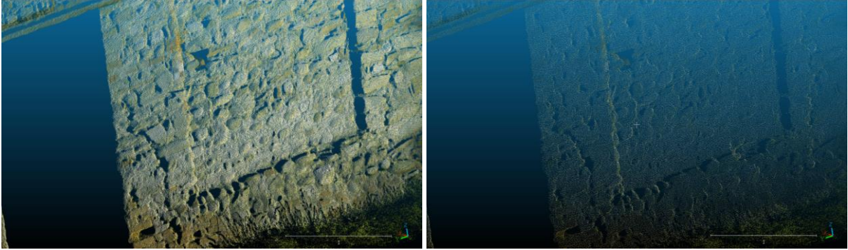
Image 33 - Before (left) and after (right) comparison of a subsampled point cloud on the CloudCompare software.
