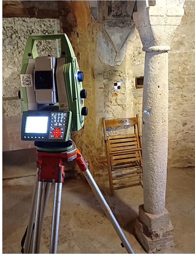
Image 17 - Total station setup at a vertex of the control network with chessboard target or point of the detail network inside the church's crypt.
