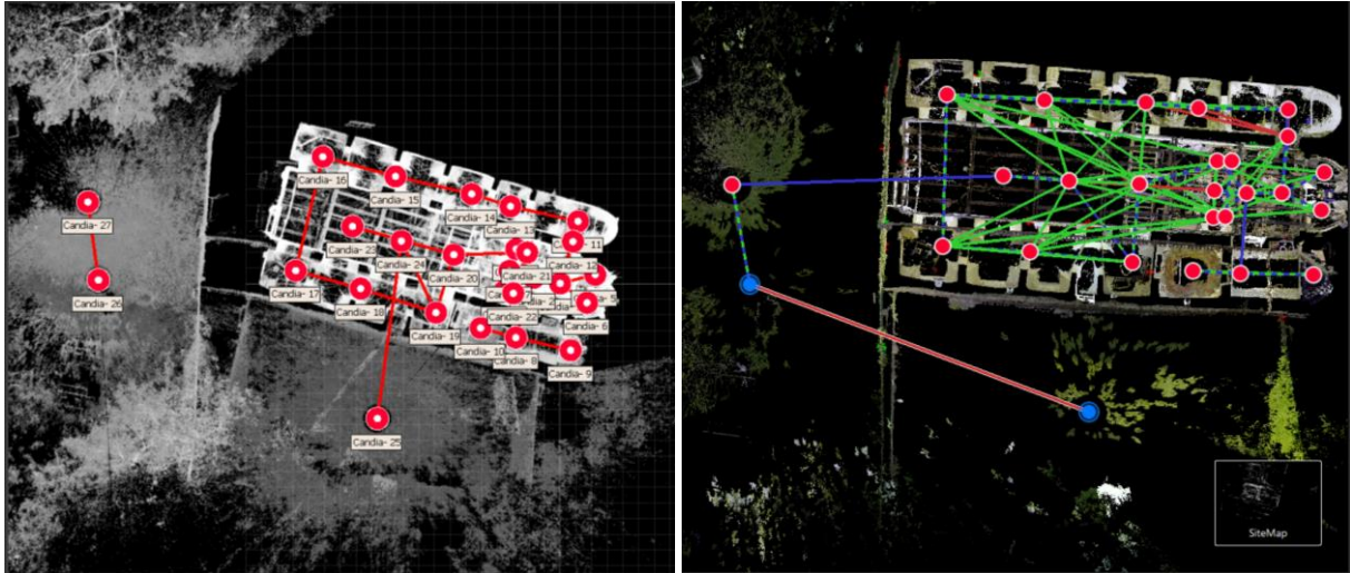
Image 24 - Upload of the laser scans to the Cyclone REGISTER 360 PLUS software (left) and Linkage of the laser scans (right).
