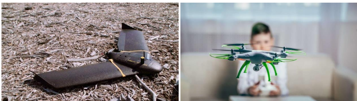
Image 15 - Fixed wing (left) and Quadcopter (right) drone Source: JOUAV. (2024, June 26). Different types of drones and uses (2024 full guide). JOUAV. https://www.jouav.com/blog/drone-types.html
