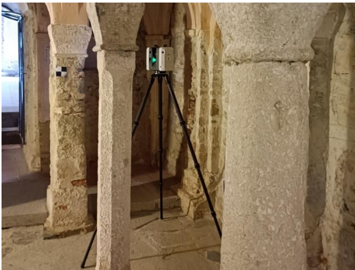
Image 18 - Positioning of the laser scanner Leica RTC360 inside the church's crypt (left), representation of laser scanner Leica RTC360 (right).
