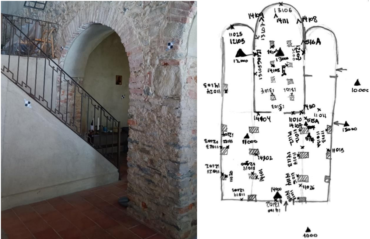
Image 16 - Example of Target Positioning in the Building for survey (left) and positioning of Total Station and Survey Points: Eidotype Diagram (right).
