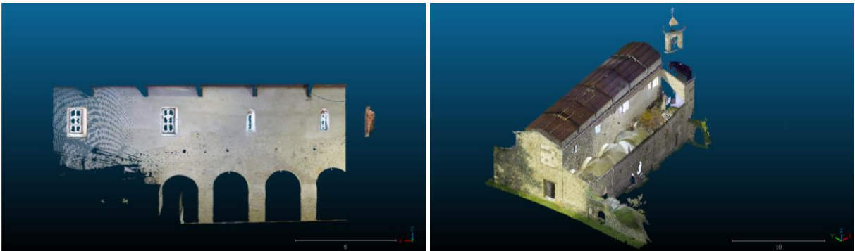
Image 36 - Enhanced laser scan point cloud with photogrammetry details (left) and final unified, subsampled, cleaned and Enhanced point cloud (right).
