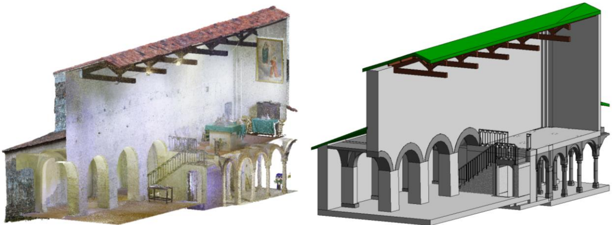
Image 54 - Side-by-Side comparison of point clouds (left) and Revit model (right).
