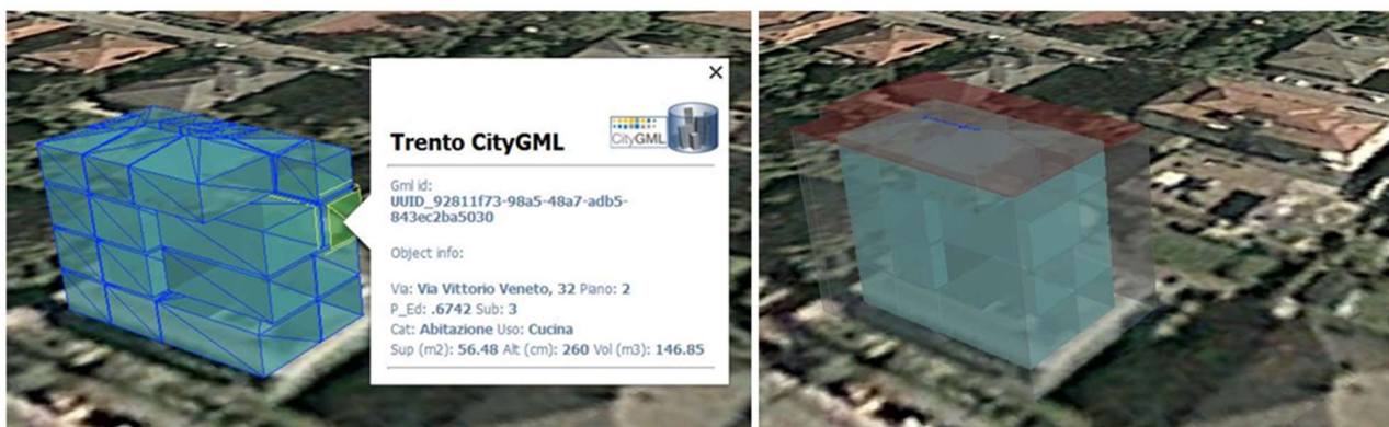
Figure 10 On the left: A three-dimensional representation of the interior of the building derived from Docfa 4 data. On the right: A combined representation of the building's façade (derived from topographic data) and interior (derived from Docfa data). Source: (Fronza et al., 2013)
