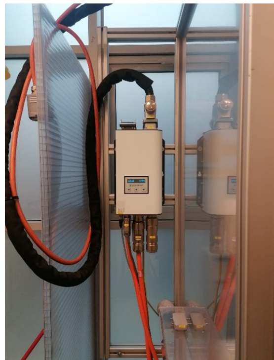
Figure 28: Power control Unit (range from 400 W to 600 W)
