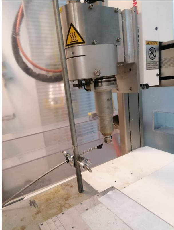
Figure 26: Plasma Source (Openair-Plasma PFW10) and Optical probe
