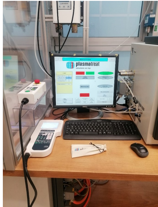
Figure 30: Process parameter display screen and control panel
