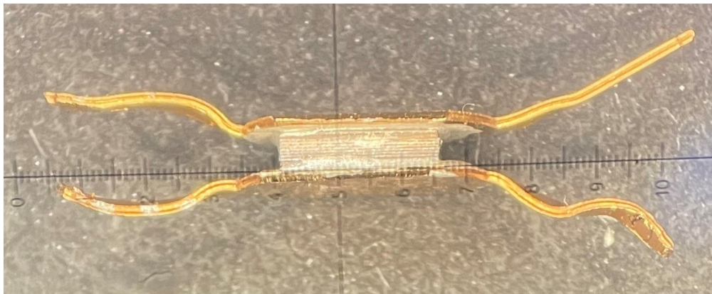
Figure 4.8: Glued sample ready to be installed in the TTO.
