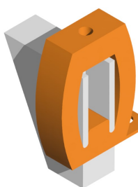
Figure 4.9: 3D CAD of the stack mold, used for 4\text{ mm} \times 4\text{ mm} tapes.
