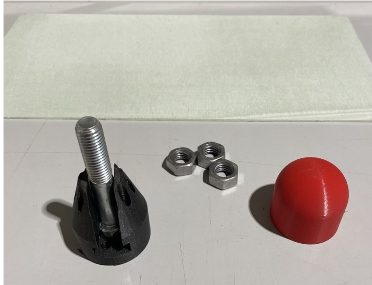
Figure 4.3: All the setup of the ball drop test: BDv1 and BDv2 (screws, nuts and holders), fiberglass pane, pipes, impact head.
