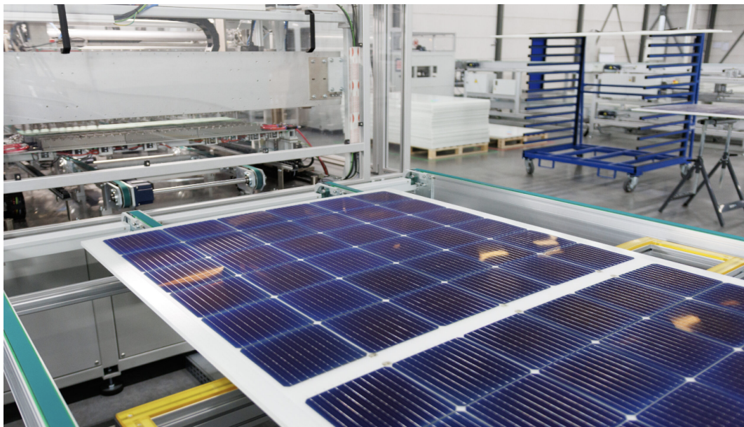
Figure A.1: Typical Solarge's polymeric panel. [16]
