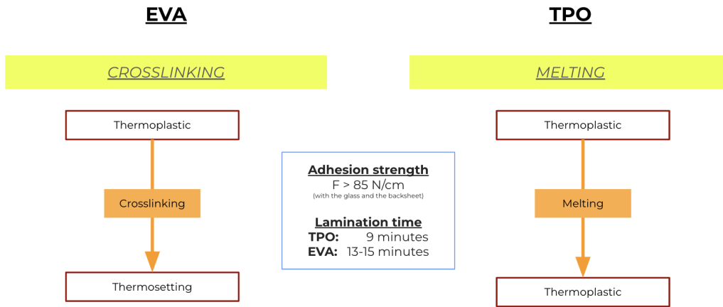
Figure C.2: Chemical cross-linking and melting for PO and EVA
