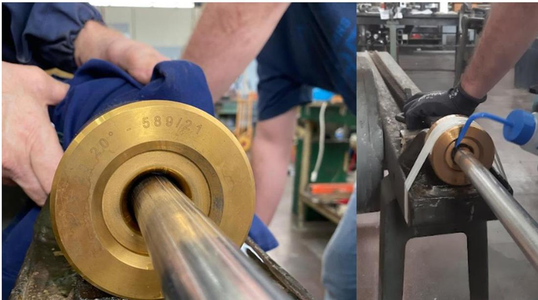
*Figure 2.1.10: Details of the wire-drawing process with one of the brass jigs used*
