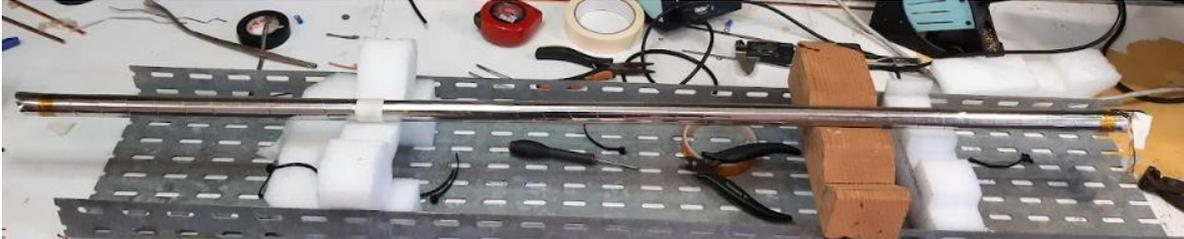
*Figure 2.1.9: Wrapped thin layers of stainless steel around the core before the jacketing process*
