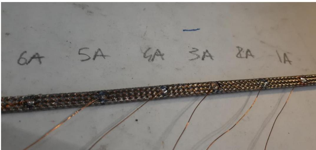
Figure 2.1.4: Picture of the soldering process for the voltage taps in the high-field region on the BRAST
