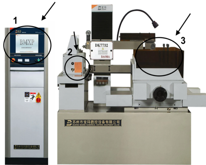
Fig. 35. Key components of the WEDM machine: Section 1 (software controls), Section 2 (coordinate display), and Section 3 (cutting area).
