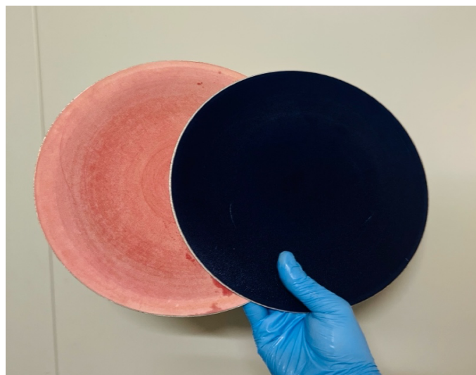
Fig. 42. Polishing pads with 1-micron (pink) and 3-micron (blue) grit sizes were used for polishing the samples.
