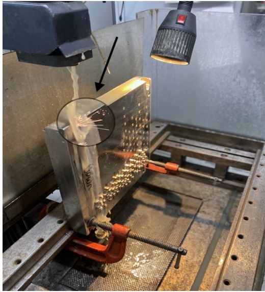
Fig. 34. Illustration of electrical sparks and the movement of water during the wire-cutting procedure.
