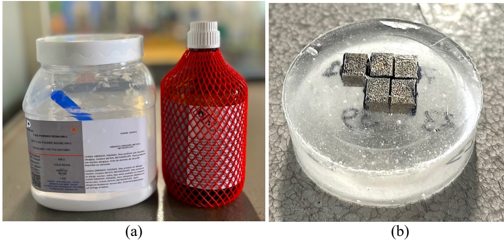
Fig. 40. (a) The acrylic resin and methyl methacrylate hardener were used for mounting the samples before the grinding and polishing process. (b) Mounted samples were removed from the mold, ready for the grinding and polishing process.
