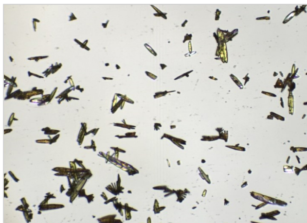
Figure 4.30: Optical microscope images of curcumin Form I (experiment COOL_KCAR)
