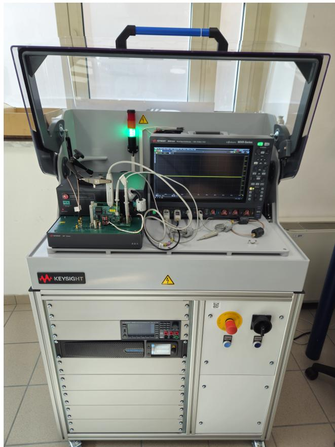
Figura 2.1: Macchina da DPT Keysight PD1500A
