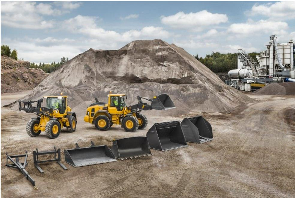
Figure 2.1: Example of different tools that can be mounted on wheel loaders for the different purposes. Picture source: [7]
