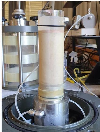
*Figure 13: Prepared sample for the test (Triaxial testing, 2021)*
