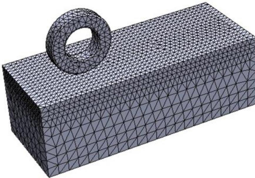
*Figure 4: 3-D mesh model tire/soil (Moslem & Hossein, 2014)*
