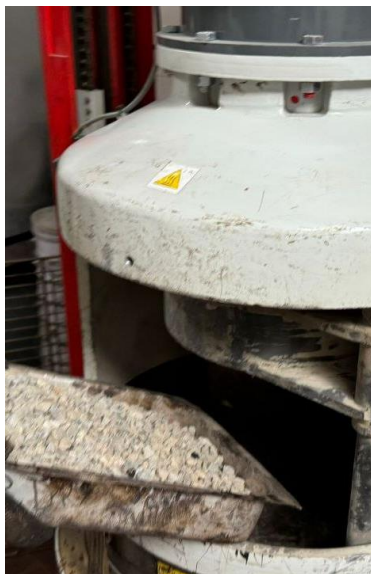
Figure 62. Pouring of coarse aggregates
