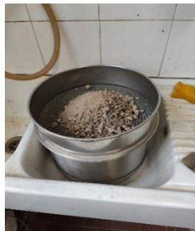
Figure 29. Preparation of aggregates and sieve for washing
