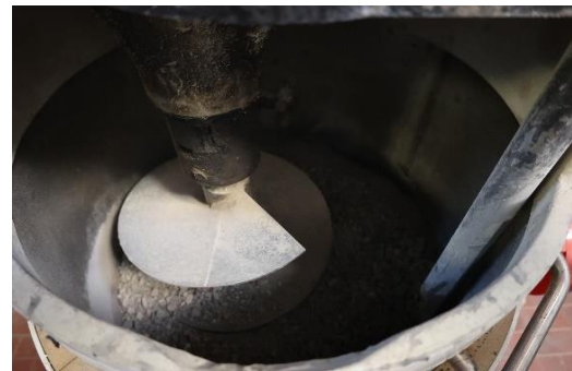
Figure 61. Mixing of aggregates only
