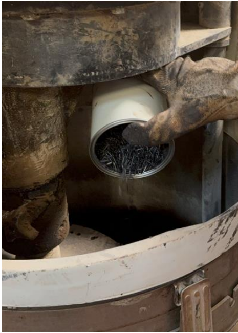
Figure 65. Pouring of fibers
