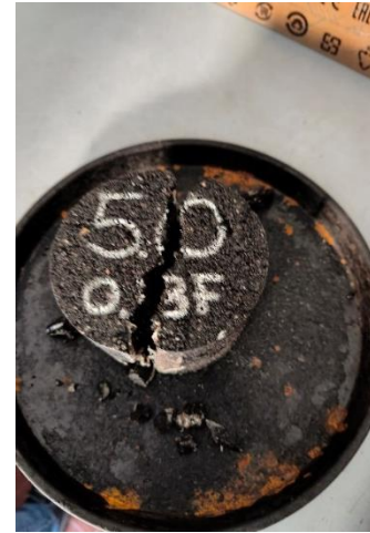
Figure 58. Example of crack in the specimen after ITS test
