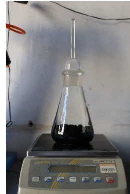
Figure 41. Weighing pycnometer with material and deaerated water.
