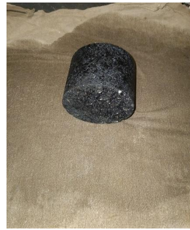
Figure 55. Surface drying of the sample for SSD, m_3
