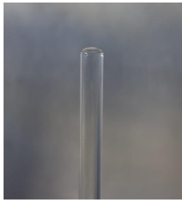
Figure 24. Convex meniscus at the end of the tube
