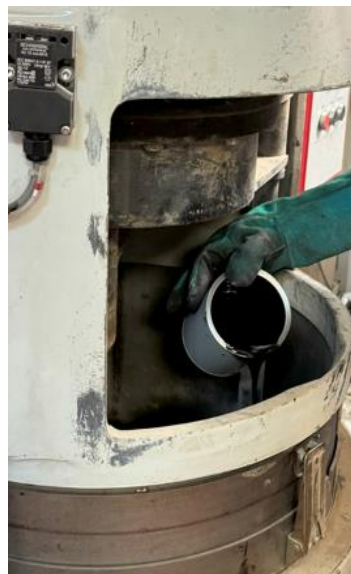
Figure 63. Pouring of virgin bitumen
