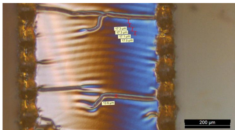
Figure 36- Microscope top view of the TiPt_S_70 sample, showing platinum tracks deposited at 70°C. The image highlights wrinkles with a consistent wavelength of approximately 17 μm. Measurements of wrinkle periodicity are displayed.
