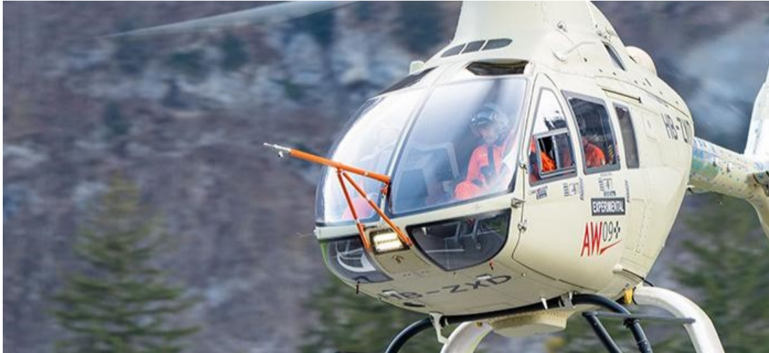
Figure 2.2: Air Data Boom assembly [ Leonardo ]
