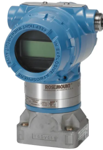
Figure 3.6: Rosemount 3051 pressure transducer. It can measure absolute or differential pressure.
