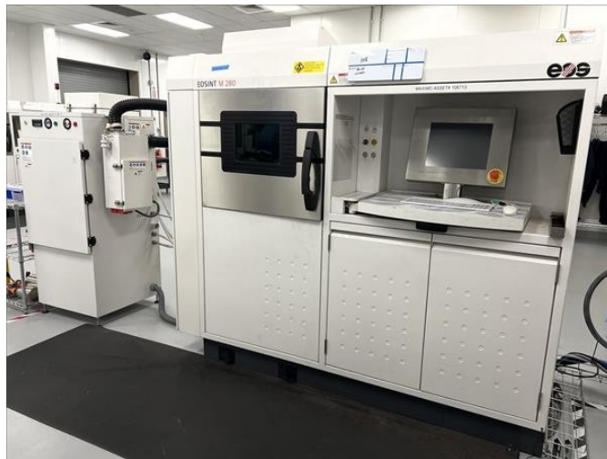
Figure 2.4: EOSINT M 280 metal 3D printer, used by Siemens Energy AM workshop
