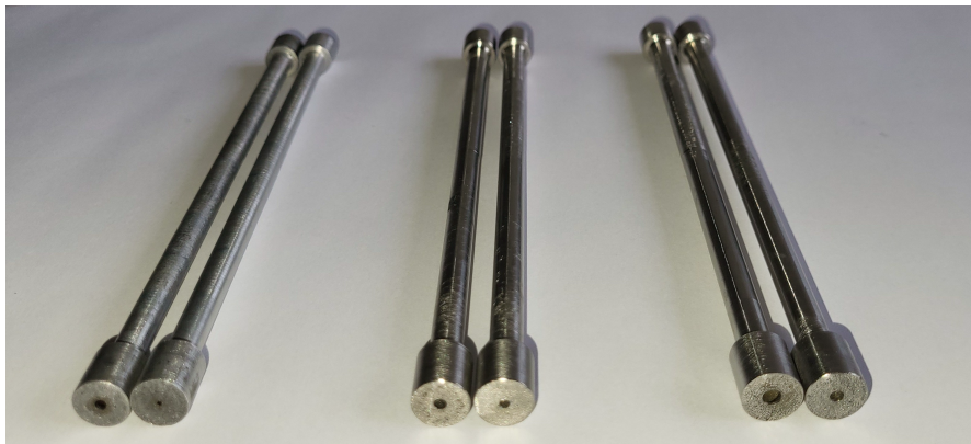
Figure 3.9: Machined test objects: Aluminum, Inconel 939 and Stainless Steel
