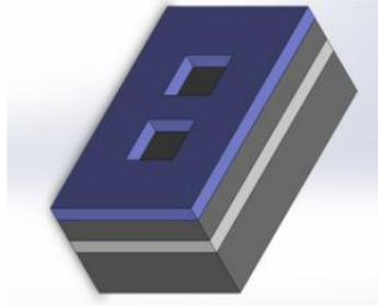
**Figure 5.3:** Second stage of e-beam lithography for silicon nanowires fabrication
