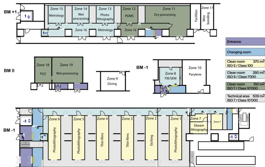
Figure 4.1: Cleanroom top view and classification at CMi, EPFL
