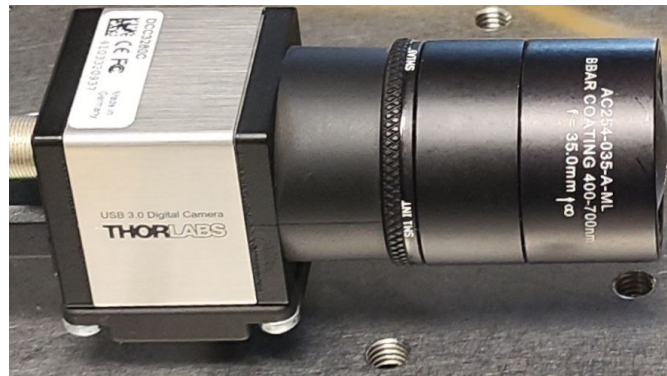
Figure 5.2: Picture of the camera and lens set-up.
