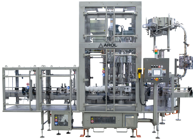
Figure 1.1. EURO PK: example of AROL capping machinery[4]
