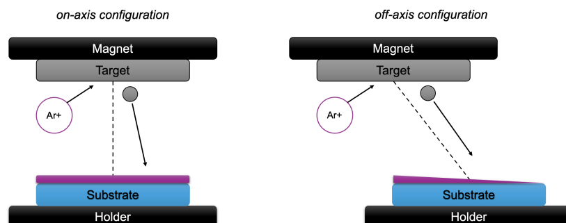
FIGURE 3.2: Magnetron sputtering: two possible configurations are available. In the off-axis configuration material can be deposited as a wedge with a thickness variation of up to a factor of 2 across a 100 mm wafer.
