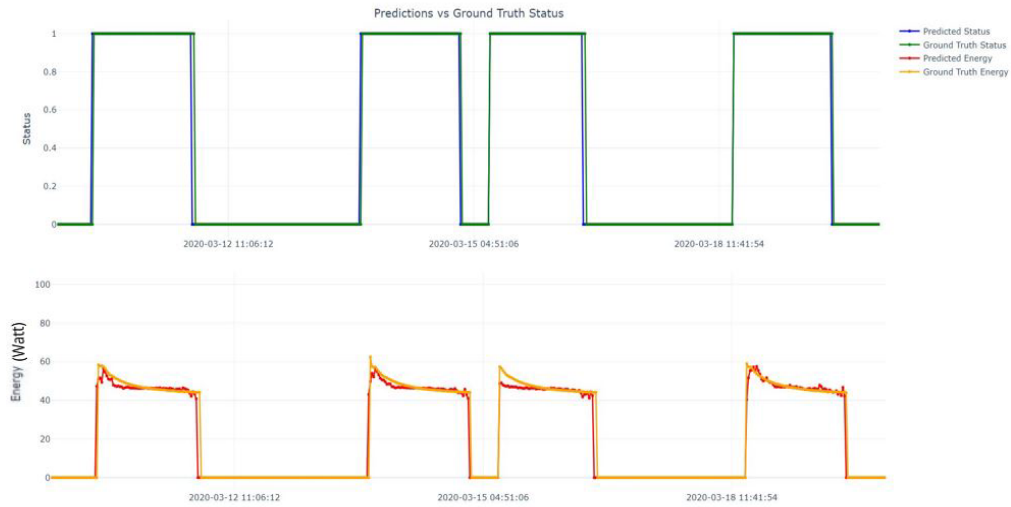
Figure 4.5: Predictions vs ground truth on Fridge - First scenario (train on SynD and test on SynD)
