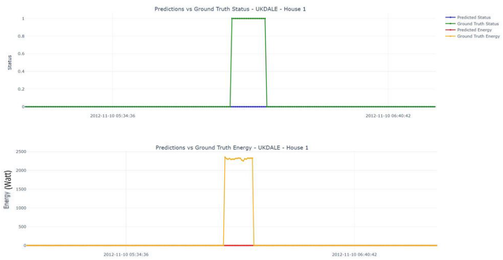
Figure 4.30: Predictions vs ground truth on Kettle - Second scenario (train on SynD and test on UK-DALE - House 1)
