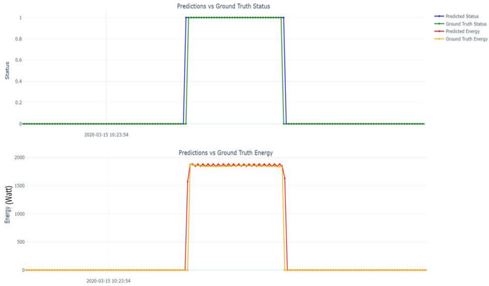
Figure 4.29: Predictions vs ground truth on Kettle - First scenario (train on SynD and test on SynD)
