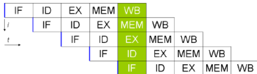
Figure 2.6: Basic five-stage pipeline in a RISC machine [19]
