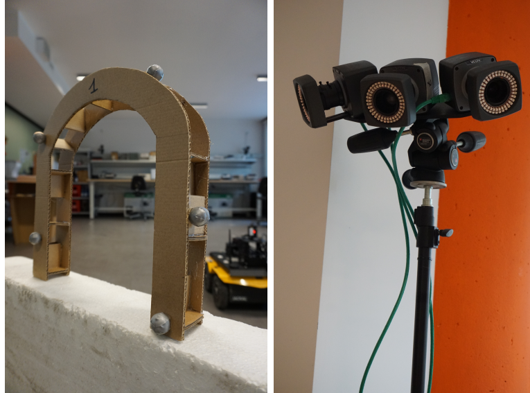
(a) Cardboard collar, with some spheres surrounded by reflective tape. (b) Three Vicon cameras.
