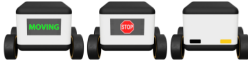
Figure 2: Three of the chosen HMI without perspective: text-based, graphical-based, dual light. (Reproduced from [3], 2021, p. 4)
