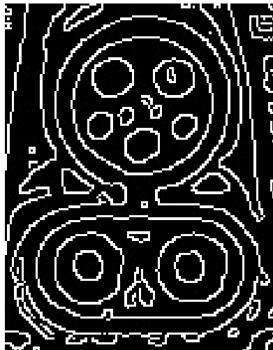
Figure 4.13: Image after Canny algorithm
