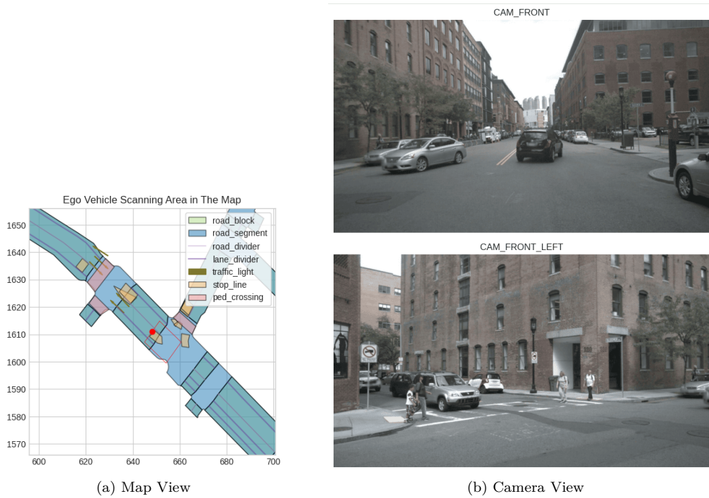
Figure 6.10: Example of turn stop. The car approaches the centre of the road to make a left turn, and yields to other vehicles by waiting on the yellow area marked on the map.
