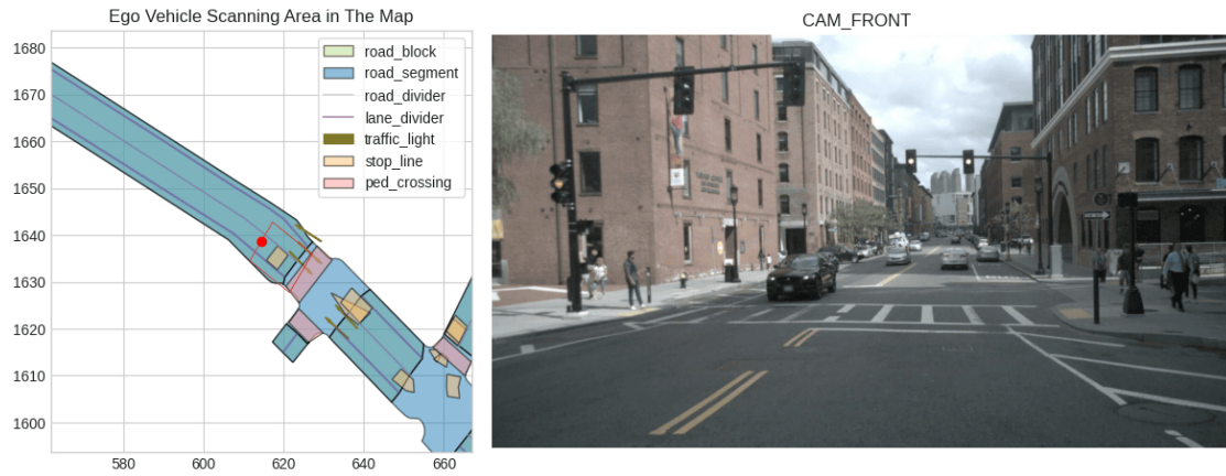
Figure 6.8: Map view and front-camera view of a frame from scene 103. The red dot marks the ego vehicle’s centre in the map view, while the red rectangle represents its scanning area. The arrows represent traffic lights. Some traffic lights intersect the scanning area but are oriented in the opposite direction, so they do not affect the vehicle. However, IsTrafficLightNearby predicate is set to Yes since the vehicle’s scanning area also intersects a stop line (yellow box) related to the traffic lights after the intersection, which are relevant for the vehicle.
