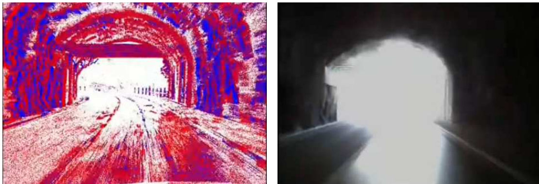
Figure 1.4: (Left) High dynamic range scene captured by a neuromorphic camera. (Right) High dynamic range scene captured by a traditional camera. Source: [4]
