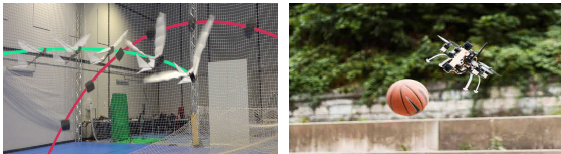
Figure 3.1: Obstacle avoidance with neuromorphic cameras, on a bio-inspired drone (left) and a quadrotor (right). Sources: [41], [37].
