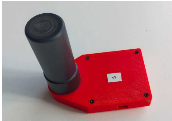
Figure 5.3: RTK GPS module for the base rover. A 3D printed case was designed to protect the module from the weather.
