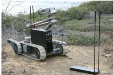
Figure 11: UGV unit carrying an APDS. [14]
