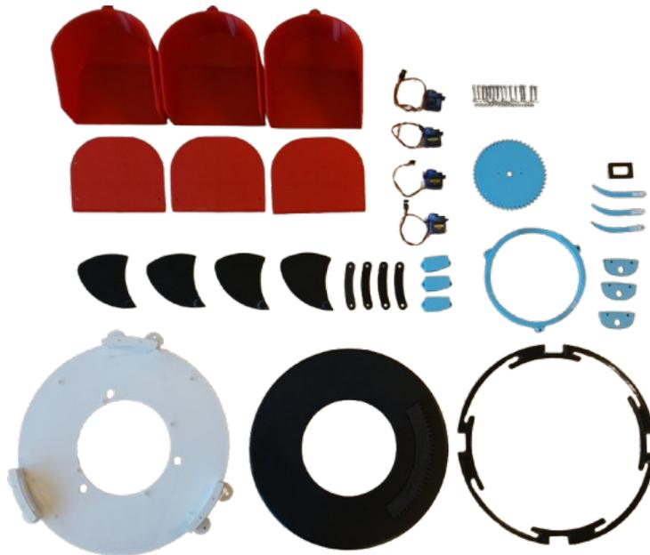
Figure 61: Disassembled Payload Dispenser.
