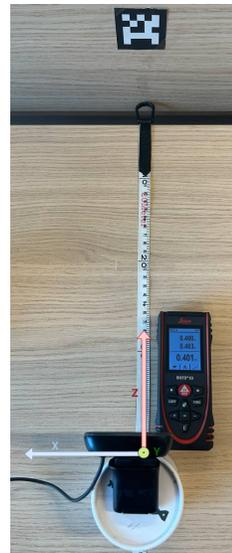
Figure 58: April-Tag Distance Testing Setup.
