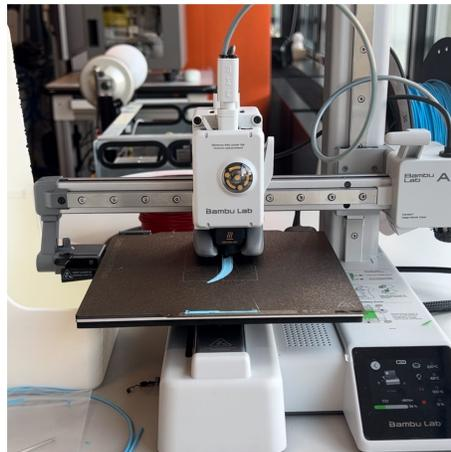
Figure 60: BambuLabA1 during the printing process of the Release Arm.
