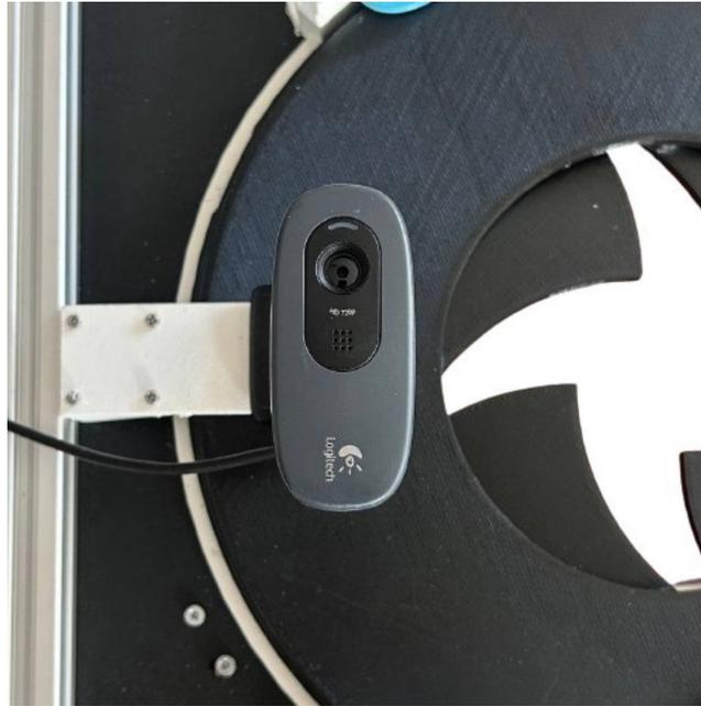
Figure 53: The cam, that is used for AprilTag detection, placed on the bottom of the payload dispenser.
